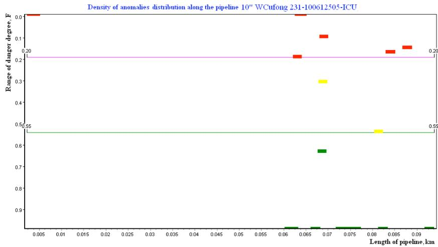
of hazard that takes into account the extent of magnetic anomalies, their amplitude and the shape of the distribution of magnetic intensity vectors over background values.
